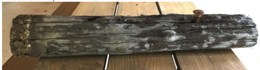
This log is most likely one end of an original tie from Myersville - circa 1896. The distance from the left end to the spike is about 2 feet, the main part of the tie would have been on the right. To the left of the spike is a spike hole the correct distance away to hold a piece of rail. It was uncovered on Main Street a few years ago. Courtesy of Myersville-Wolfsville Area Historical Society.
